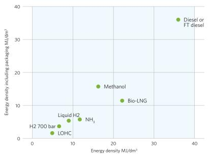
**Figure 37. Energy Density of Different Fuel Types**
