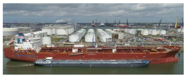
Figure 51. Barge-to-Ship Methanol Bunkering at the Port of Rotterdam
