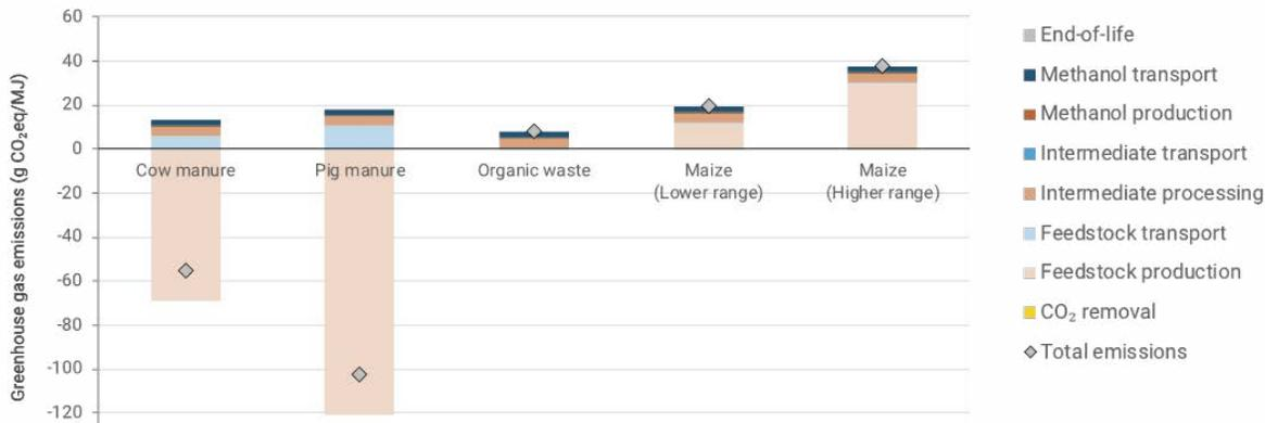
Figure 9: Methanol from Biomethane Supply Chain Emissions Depend on Feedstock
