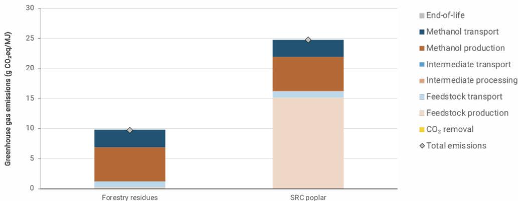
**Figure 10: Methanol from Wood Supply Chain Emissions Depend on Type of Biomass**
