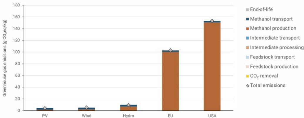
Figure 12: E-Methanol Supply Chain Emissions Depend on Source of Electricity
