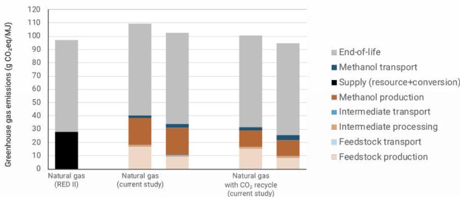
Figure 3: Emissions from the Production of Methanol from Natural Gas
