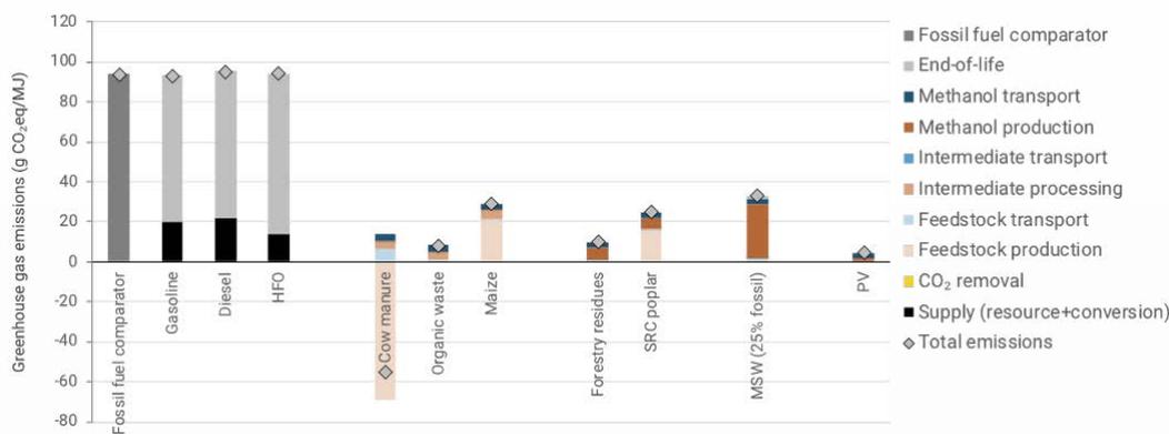
**Figure 8: Carbon Footprint of Renewable Methanol and EU RED II GHG Emission Reduction Thresholds**
