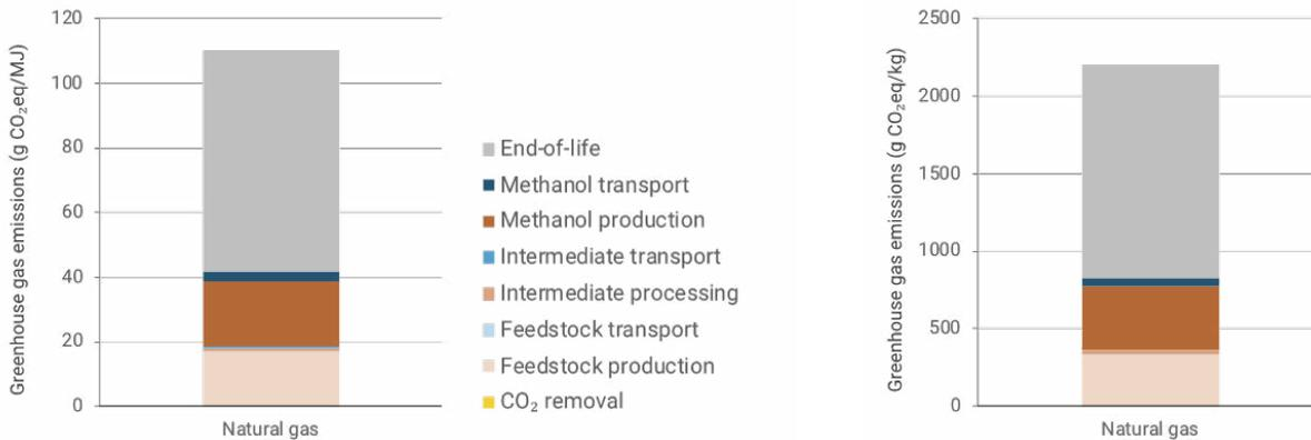
Figure 4: Methanol from Natural Gas Full Lifecycle Emissions on Energy Basis (left) and Mass Basis (Right)
