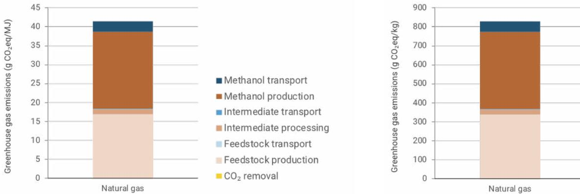
Figure 5: Methanol from Natural Gas Supply Chain Emissions (ie. Well-to-Tank)
