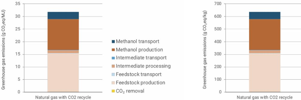
Figure 6: Methanol from Natural Gas with CO<sub>2</sub> Recirculation Supply Chain Emissions (ie. Well-to-Tank)
