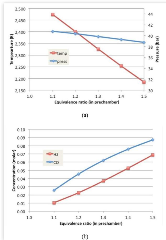
operation determines where it is most advantageous to operate the prechamber.
