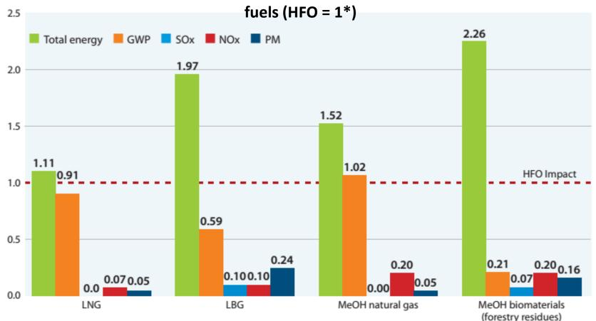
\*Energy input and impacts are considered from a well to propeller perspective and apply to the fuel used for transporting one ton for one km with a RoRo ship. LNG figures assume 4% methane slip, as reported by the manufacturer. Source: Brynolf et al, 2014
