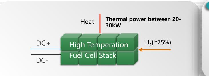
We use "high-temperature fuel cell stack", the temperature of the heat exchanger is about 140 degrees, the heat energy can be fully utilized to heat the lithium cell and the car.
