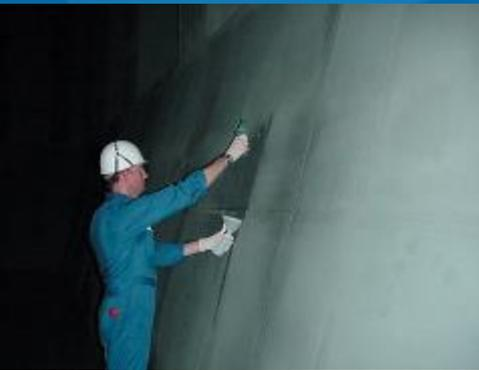
Methanol Wall Wash Test
