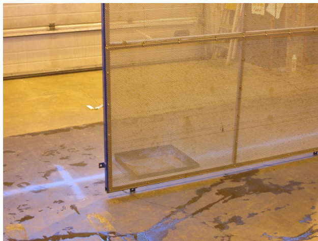
Figure 3. Perforated sheet in front of methanol fire.
