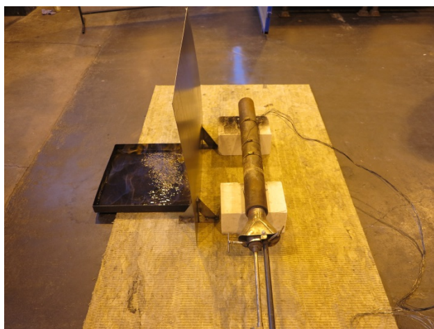
Figure 10. Hot surface and 75 cm steel sheet in front of fire.
