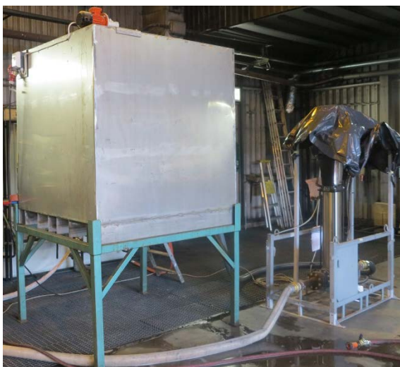
Figure 5. Water tank with premixed foam and pump (left) for the water-spraying system.
