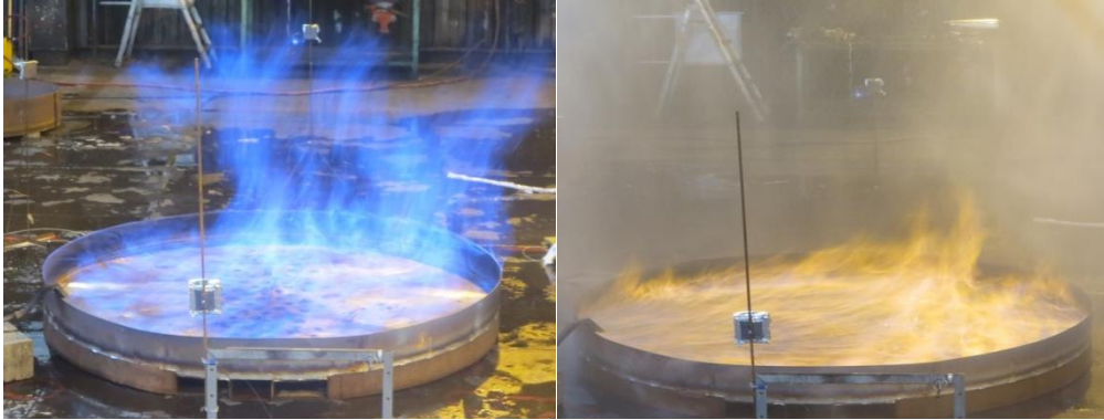
Figure 1. Flames from a methanol pool fire, free-burning and exposed to water-mist.
