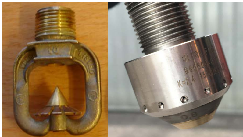
Figure 6. Water spray (left) and water-mist (right) nozzles used in the extinguishing tests.
