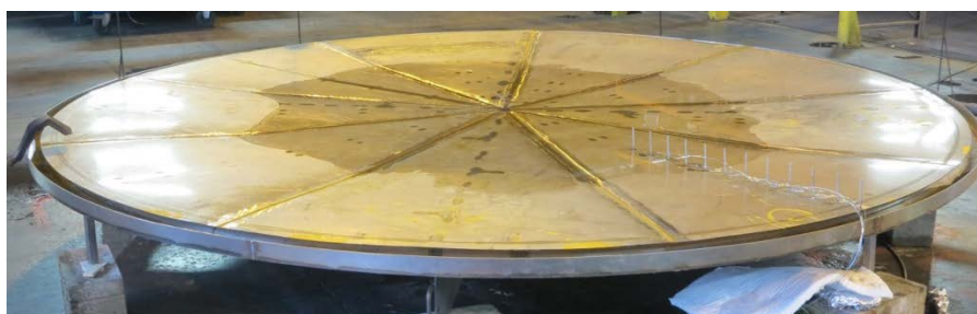
Figure 3. The conical bottomed tray (Ø4.0 m) with an about Ø2.4 m methanol pool (90 l).
