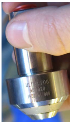
Figure 7. High pressure water-mist nozzles used in the fire extinguishing tests.
