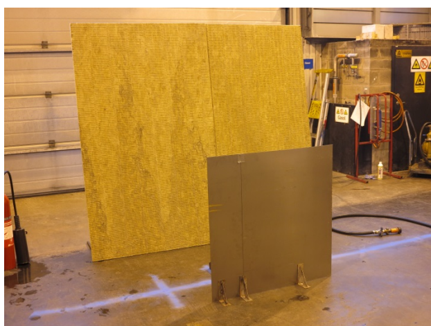
Figure 7. 100 cm steel sheet in front of fire. Insulation board positioned behind fire to reduce reflections.
