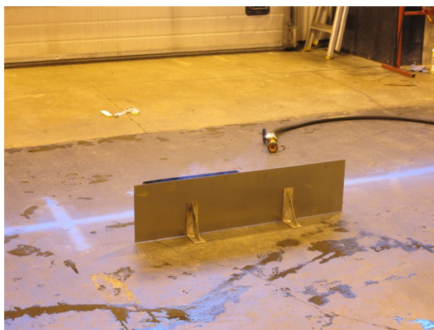
Figure 4. 25 cm steel sheet in front of fire.
