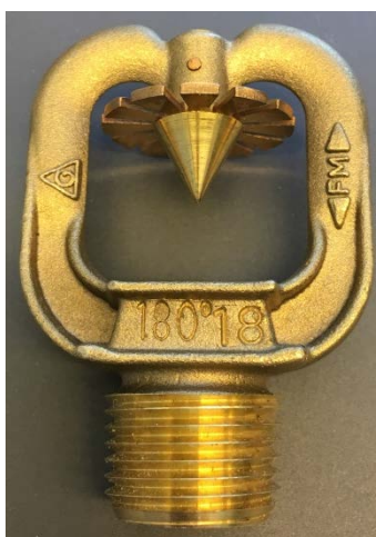
Figure 4. Water spray nozzle used in the fire-extinguishing tests.
