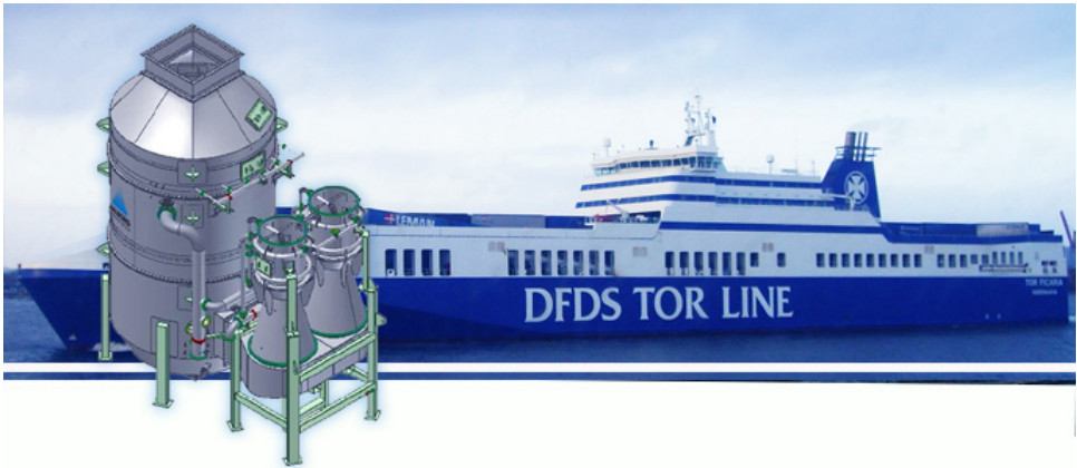
Figure A-4. Ficaria Seaways Equipped with Presumably World's Largest Retrofit Scrubber in 2009 (Source: Alfa Laval)
