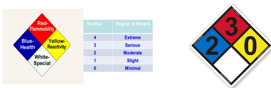
Figure 6-1. NFPA chemical hazard labels, with methanol label on the right
