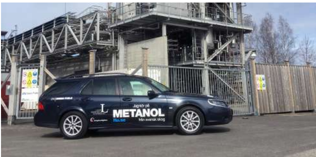
Figure 44. Swedish car powered by an M56 mix (56% methanol in gasoline) with bio-methanol from the LTU Green Fuels plant (in the background)
