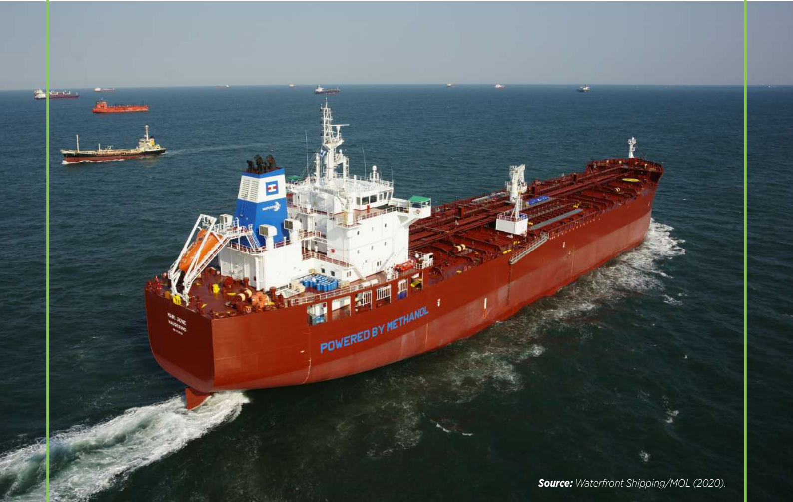
Figure 14. Ocean-going vessel powered by methanol
