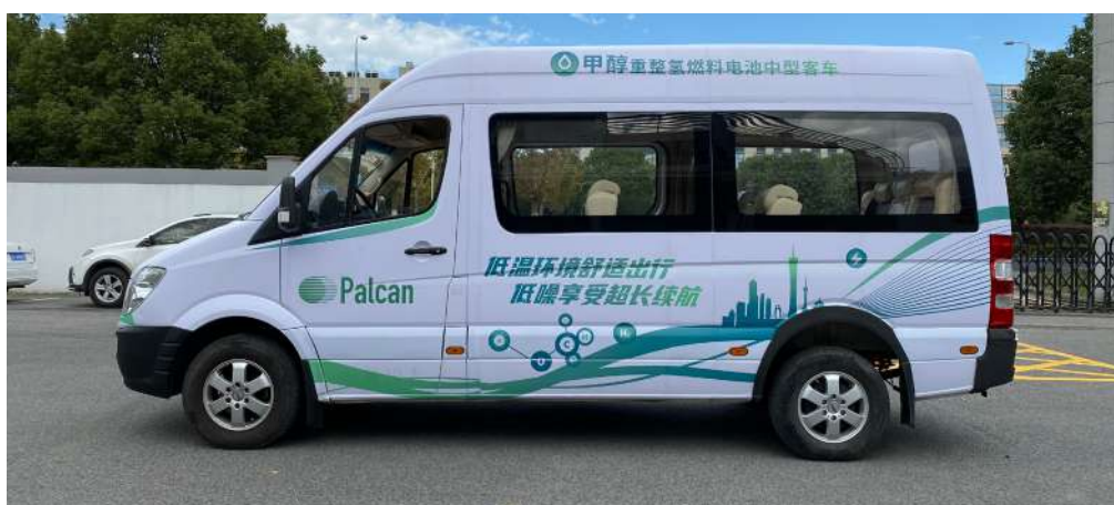
Figure 12. Palcan hybrid methanol reformer/proton-exchange membrane fuel cell passenger bus in China
