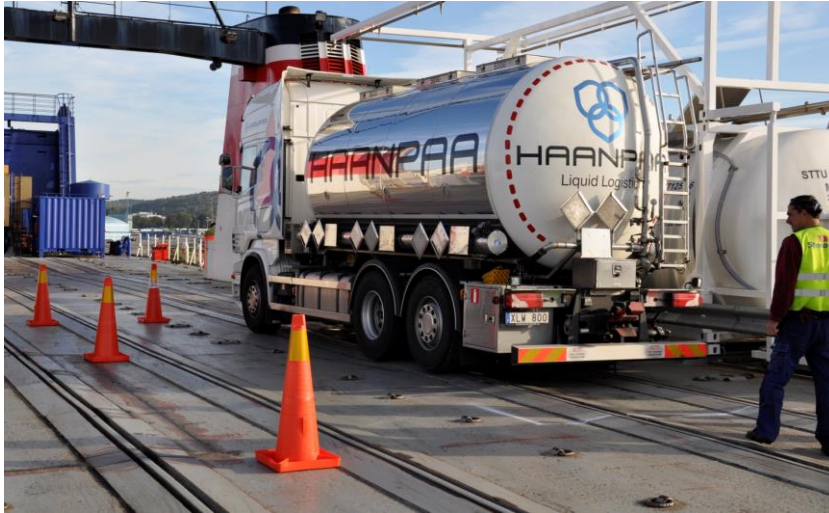
Figure 22 Bunkering methanol from a tanker truck on the Stena Scanrail for the SPIRETH project
