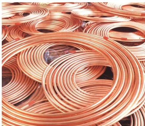
Copper alloys are used primarily for heat transfer in methanol service (titanium alloy Ti-6Al-4V, a superior tube material in sea water and hydrocarbon applications, is incompatible in methanol service). Copper alloy designations are listed below using the Unified Numbering System (UNS) for Metals and Alloys. Unlike ASTM, UNS is not a specification. Various categories of copper family of alloys are listed as follows:
